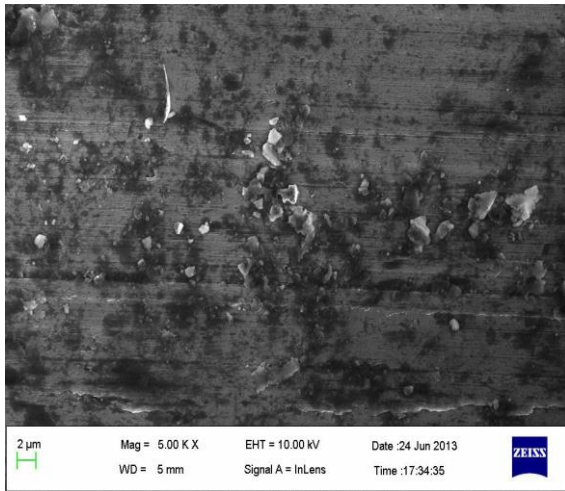
Fig 9: SEM Image [Al7075+2%SiC]
