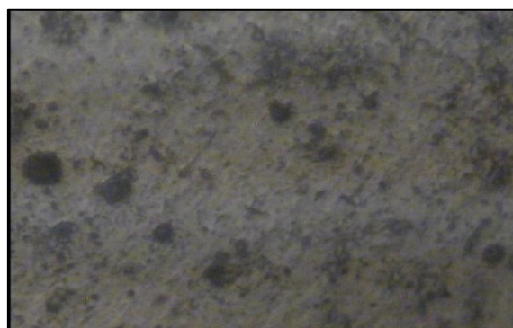
Fig 2: Optical Micro. [Al7075+0.5%nSiC]
